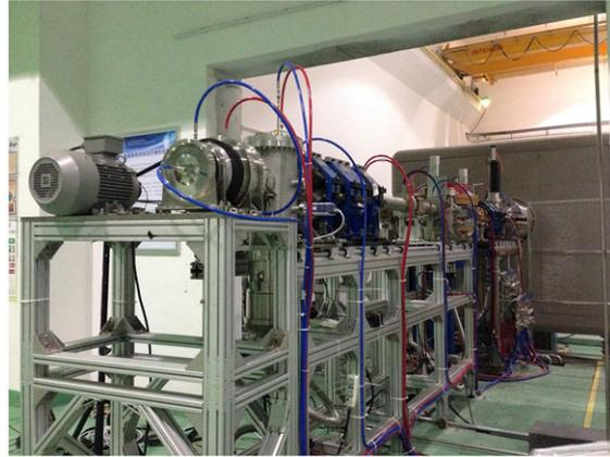
**Figure 2.** High-power rotating tritium target of HINEG-I.
