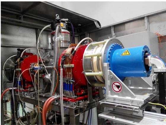
**Figure 1.** Ion source and low energy beam transport of HINEG-I.
