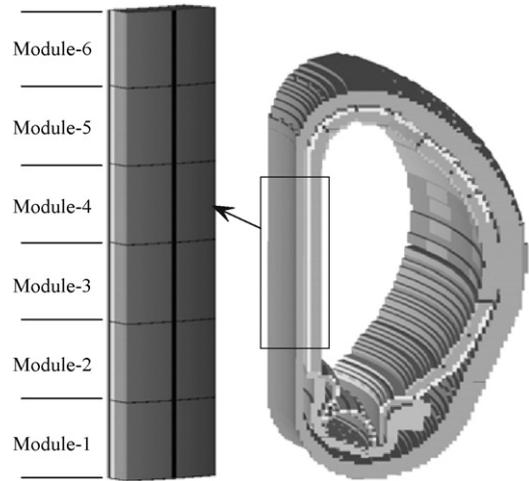
Fig. 4. Inboard blanket modules of ITER 3D model.
