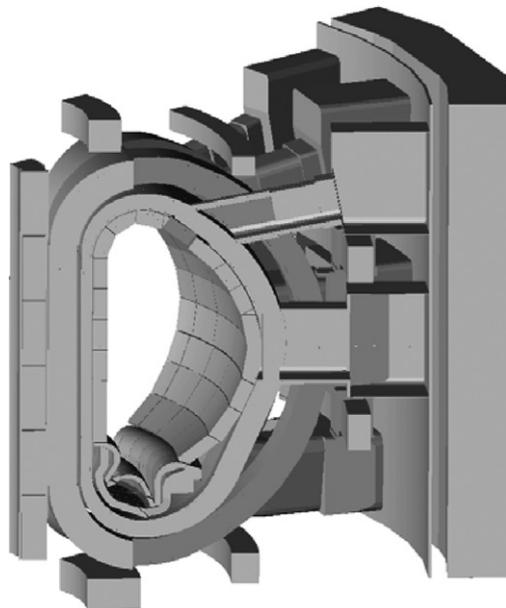
Fig. 1. ITER 3D model created in CATIA.
